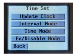
2. Press the **EN/DISABLE MODE** button, which takes you to the next screen as shown below, to enable and start the interval program you just set.
