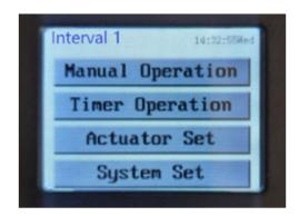
Note: At the top of the screen, it says "Interval 1", this means the program is enabled and running.
